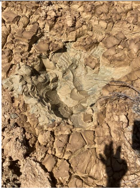
Figure 20: PL2 Wet Tails showing crusting
